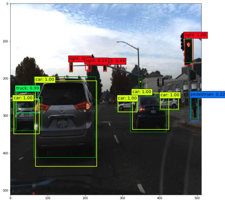
Figure 4.4: Predictions of the SSD-7 on an image of the Udacity[24]/Roboflow[5] dataset
