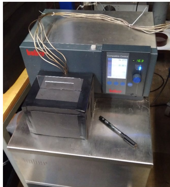
Picture A 2: Insulated lid for T-history experiment
