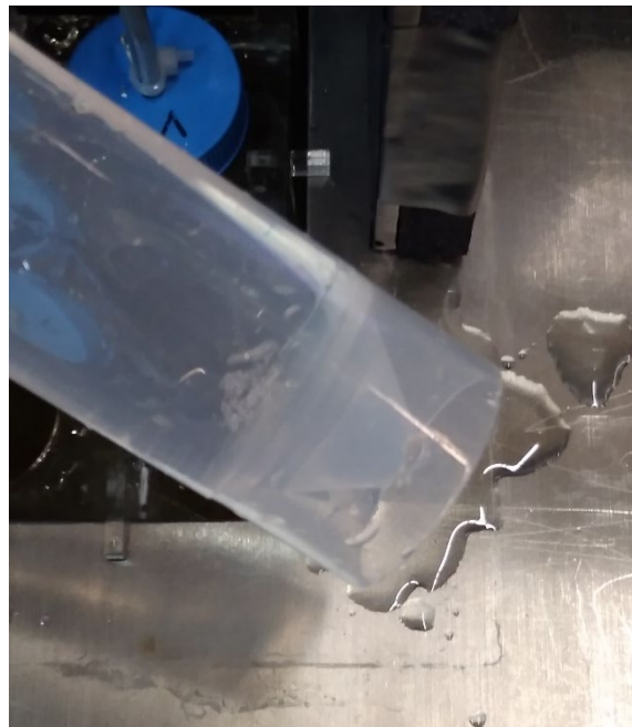
Picture A 12: Solid crystals at bottom of 23.3% NaCl-solution.
