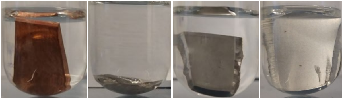
Figure 5 shows examples of the performed material compatibility tests at day 1. From left to right: copper, steel, stainless steel, aluminum in n-Decane.
