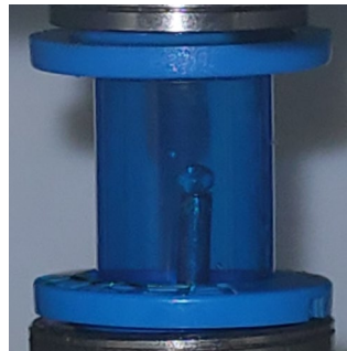
Figure 13: Bubble on inlet temperature sensor.
