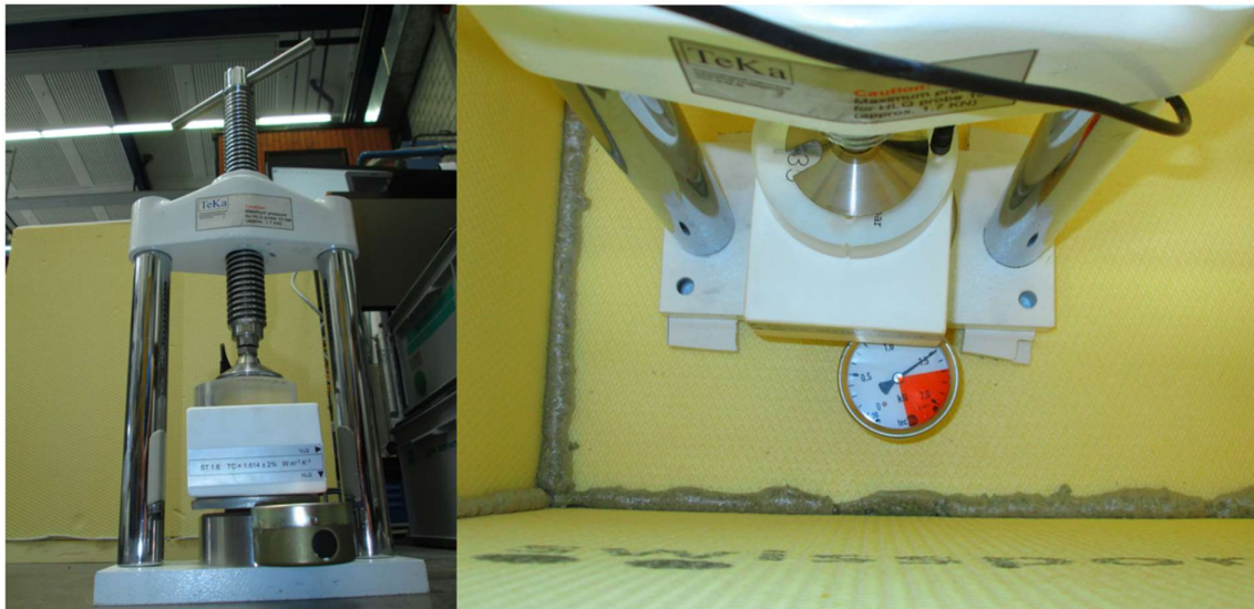
Figure 21: TeKa clamp with HLQ probe and reference block (left), placed in guard box (right)
