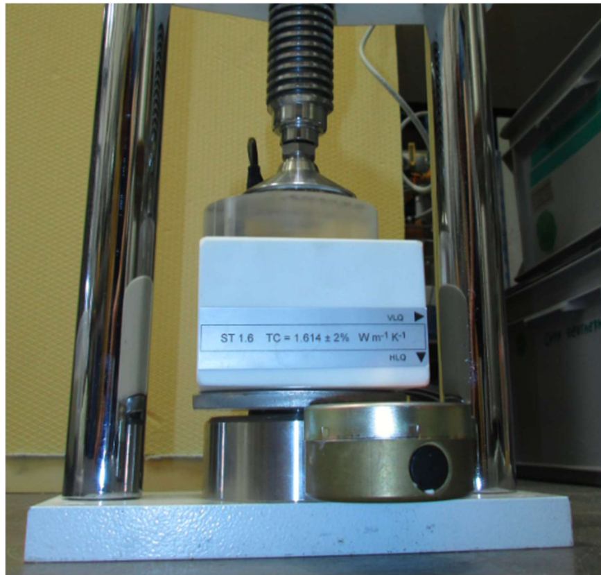
Figure 18: TeKa ceramic sample material with HLQ probe in pressure clamp
