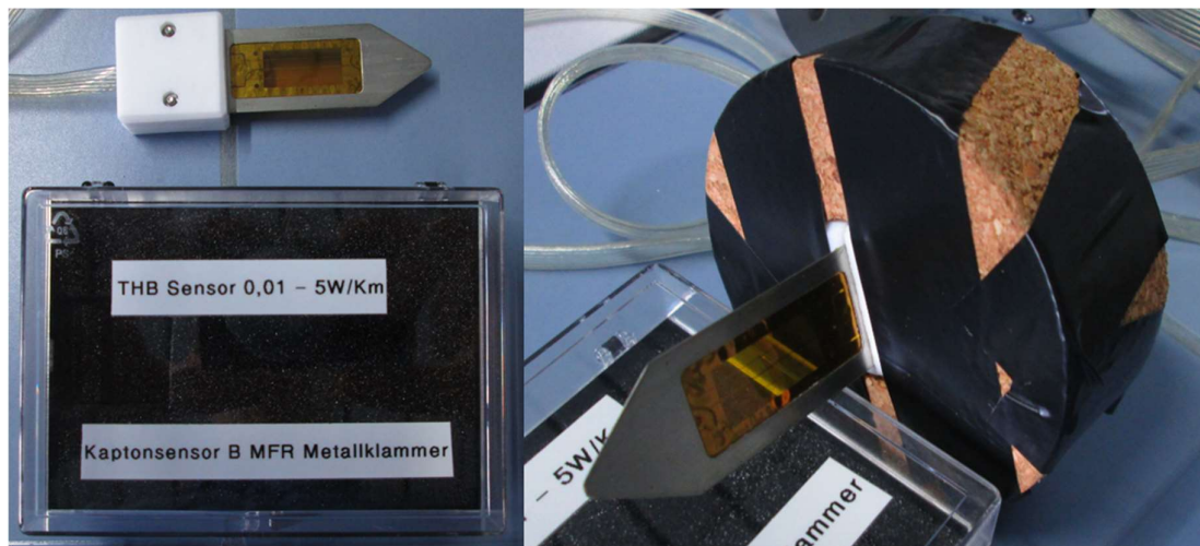
Figure 25: THB sensor used to measure PQS sample (left), sensor fixed to cork donut for support (right)
