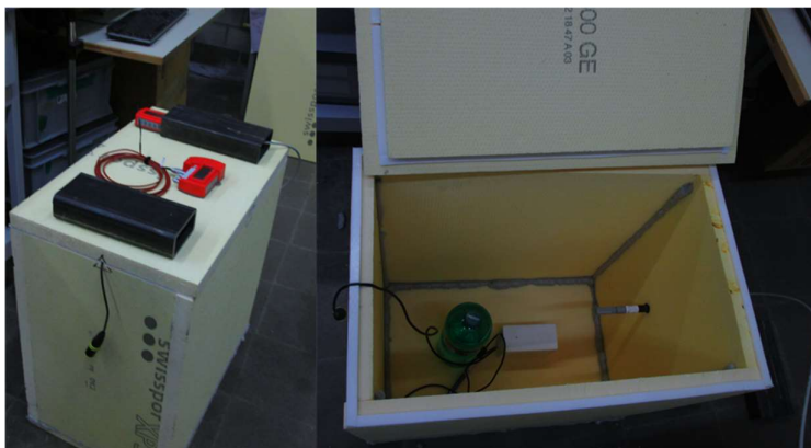
Figure 16: Guard box with temperature and humidity monitors
