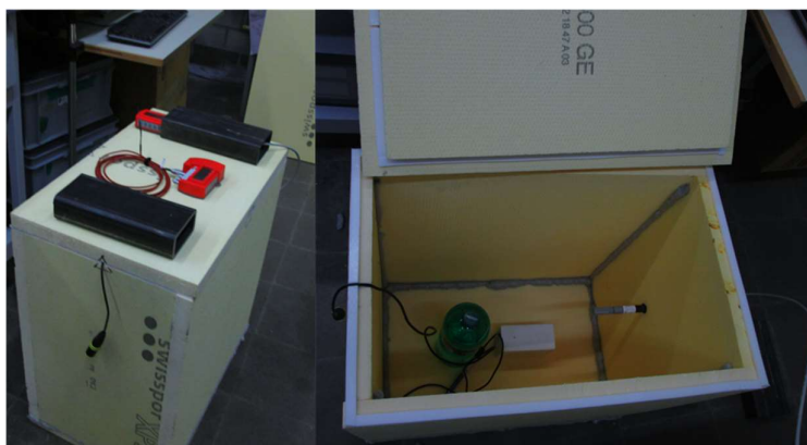
Figure 16: Guard box with temperature and humidity monitors
