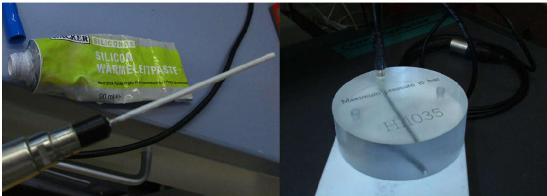
Figure 17: TeKa VLQ sensor with thermal paste (left) and HLQ sensor (right) on a planar surface.
