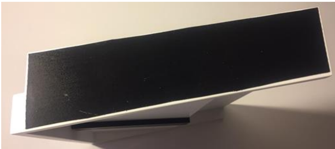
Figure [40]: Micro Velcro from side view of 8° angled hand support
