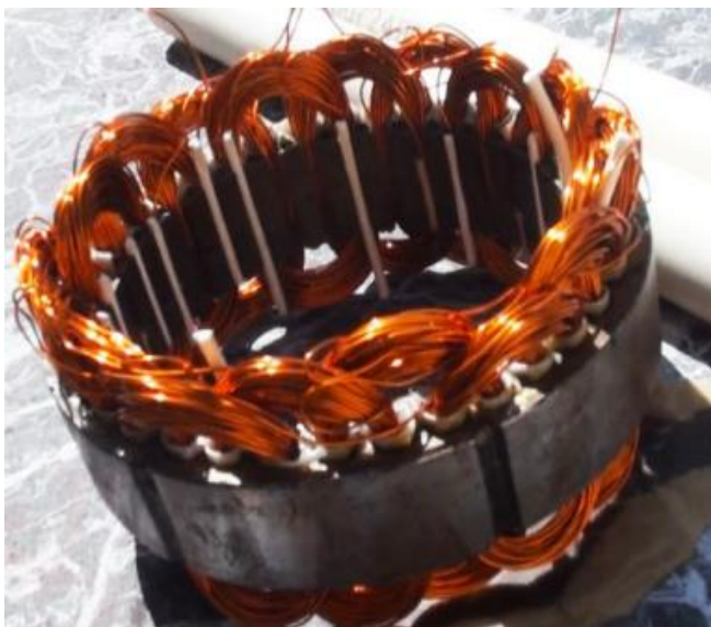
Figure 75 Rewound car alternator
