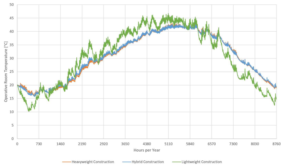
Figure 7: TCY of Construction Types without Solar Protection and Nighttime Ventilation
