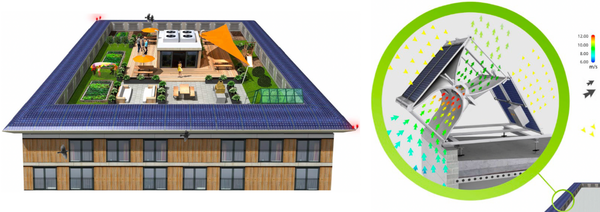
Figure 7: Concept of the building with 'WindRail' diffuser augmented wind turbines in combination with PV panels on the roof from http://www.anerdy.com
